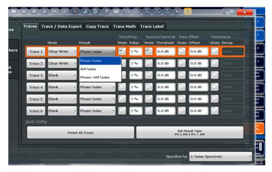
In the trace menu, users can assign traces to phase noise and/or amplitude noise measurements. They can also select whether they want spurious removed or traces smoothed or whether the traces should be displayed in the persistence mode.
