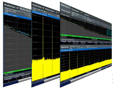
Users can switch between the spectrum analyzer and phase noise analyzer measurement channels or view both simultaneously
