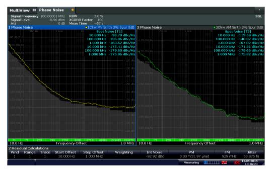
The R&S\*FSWP can measure phase noise and amplitude noise simultaneously. The results can be displayed in separate windows or together in one window (gray area: correlation gain of the R&S\*FSWP, green trace: amplitude noise, yellow trace: phase noise).
